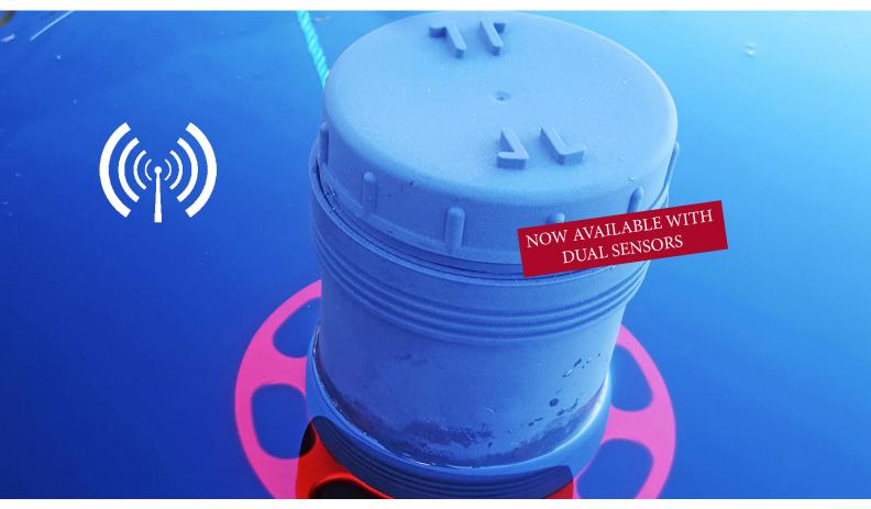
Guardian is floating buoy equipped with optical sensors and unit for data processing. Data is transmitted through GSM to a cloud-based storage and web page for further data management.
